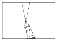
Figure 8. Lubricating nailer via air inlet.
